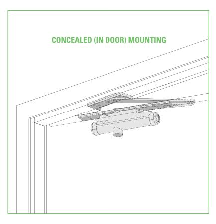
The concealed 330 is designed to mount in a 1 3/4" interior door. The double lever arm provides superior door control and the choice of finishes and arm functions meet virtually all architectural requirements.
